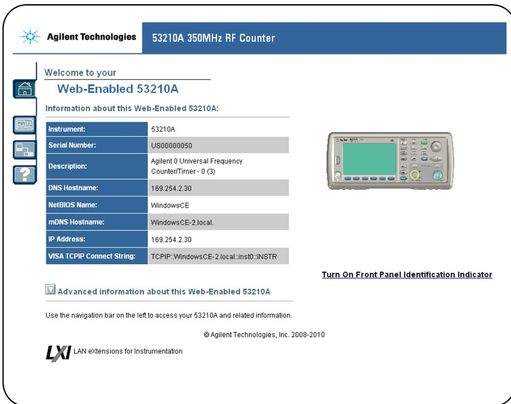
The screenshot displays the web interface for the Agilent 53210A 350MHz RF Counter. The page features a navigation bar on the left with icons for Home, Information, Settings, and Help. The main content area includes a welcome message, a table of instrument details, a photograph of the device, and a link to advanced information.
